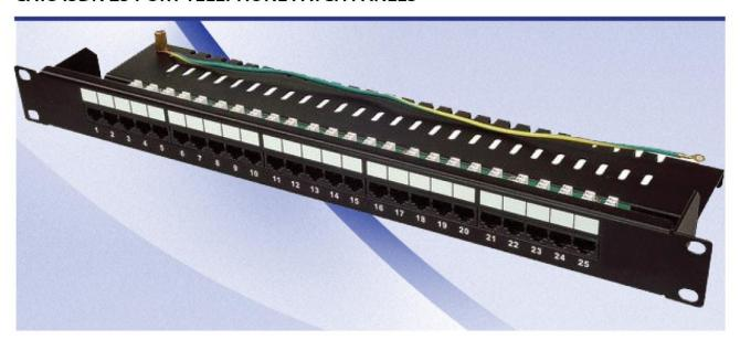
The Cat3 / ISDN telephone patch panel is a high-density telecommunication panel with 25 Standard RJ-45 Jacks. Print circuit board together with high quality components ensures the Cat3 performance. All ports are numbered. It offers a simple and economical way to connect the telephone system or the telephone backbone. The panel is available in 1U height.
